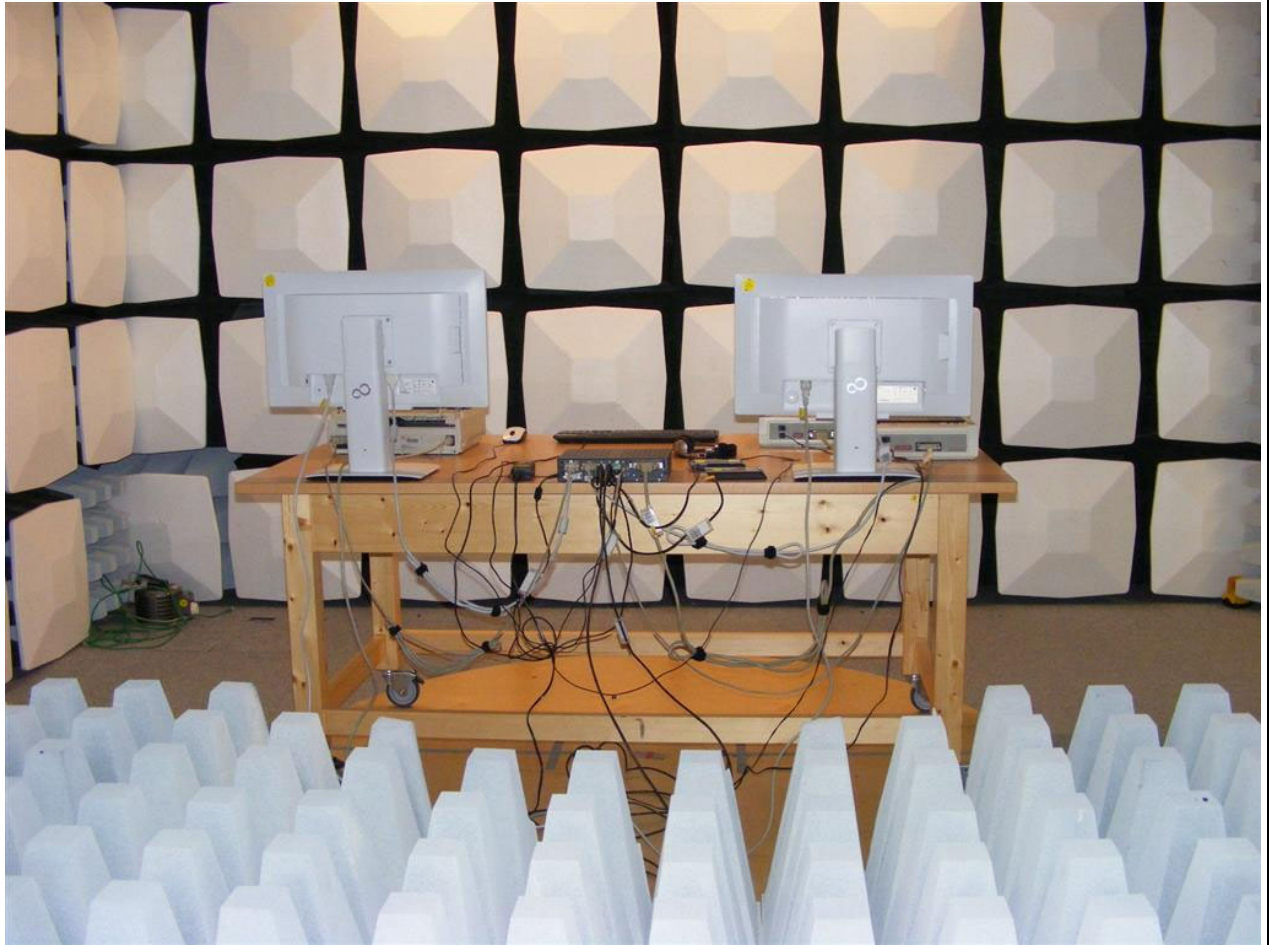
Figure 2 : Test set up Radiated Disturbance Emission - rear view
