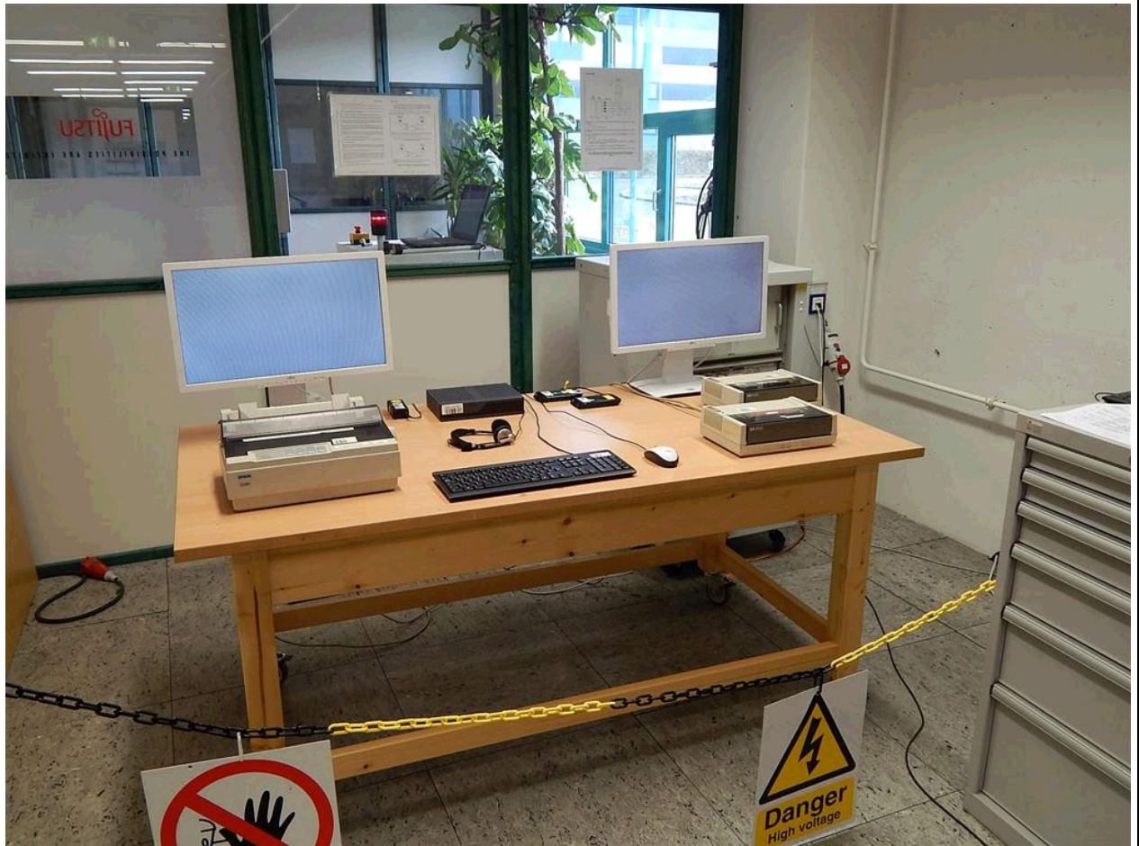
Figure 1 : Test set up for Surge Immunity - front view
