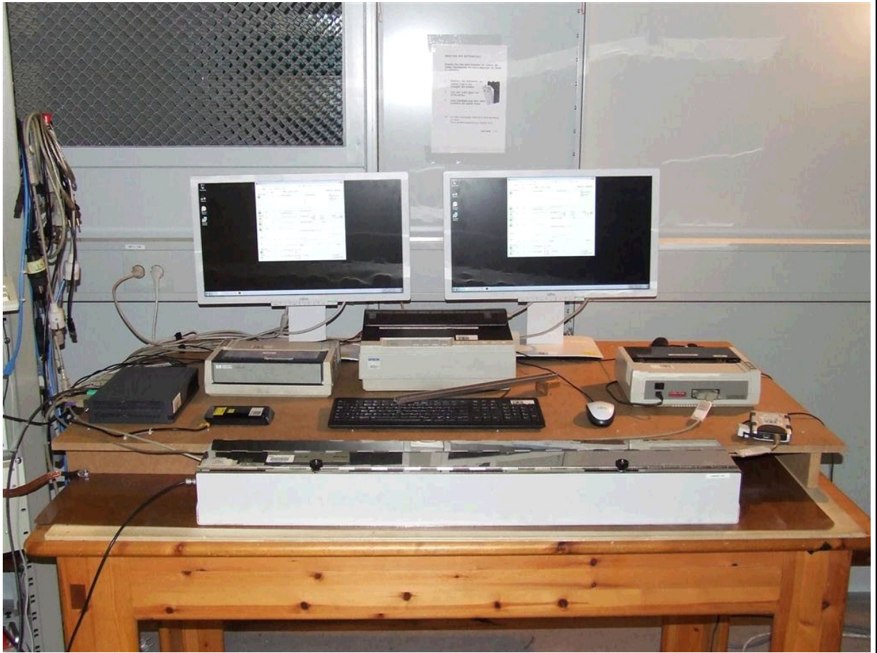
Figure 1 : Test set up for Electrical Fast Transient Immunity, Burst - front view
