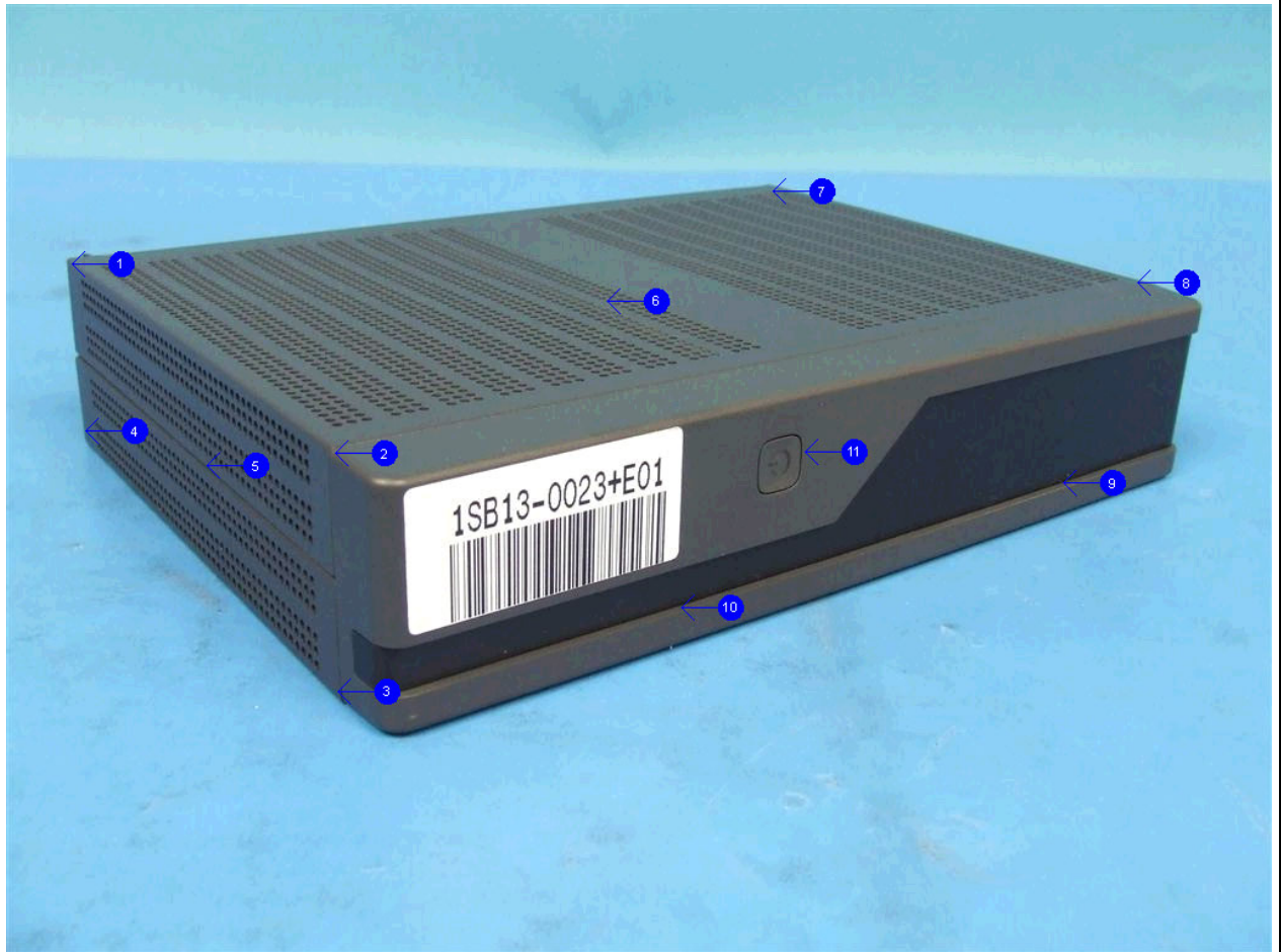
Figure 3 : Test set up for Electrostatic Discharge Immunity - test points front. Air discharge.
