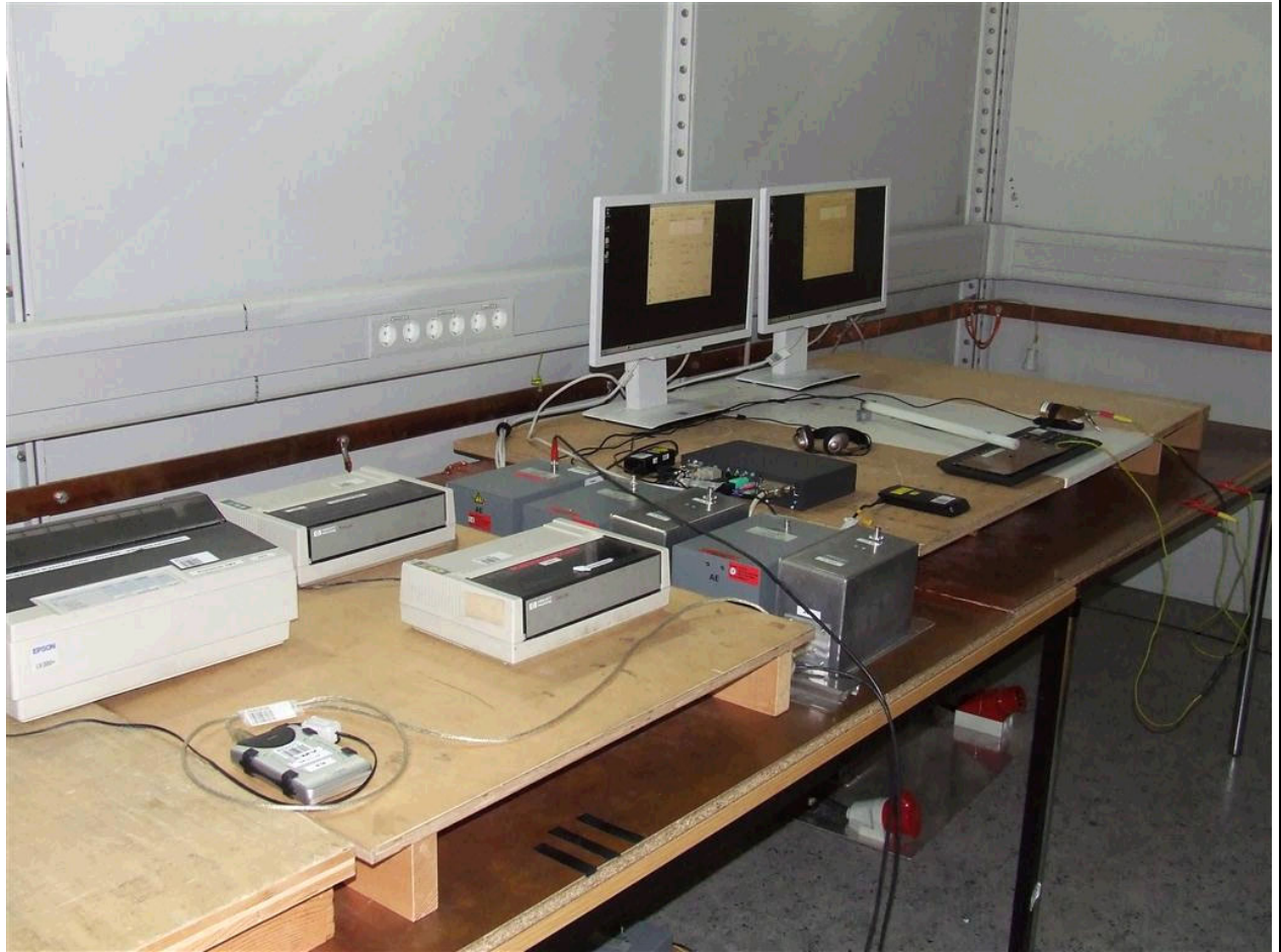
Figure 2 : Test set up for Conducted Disturbances Immunity - side view
