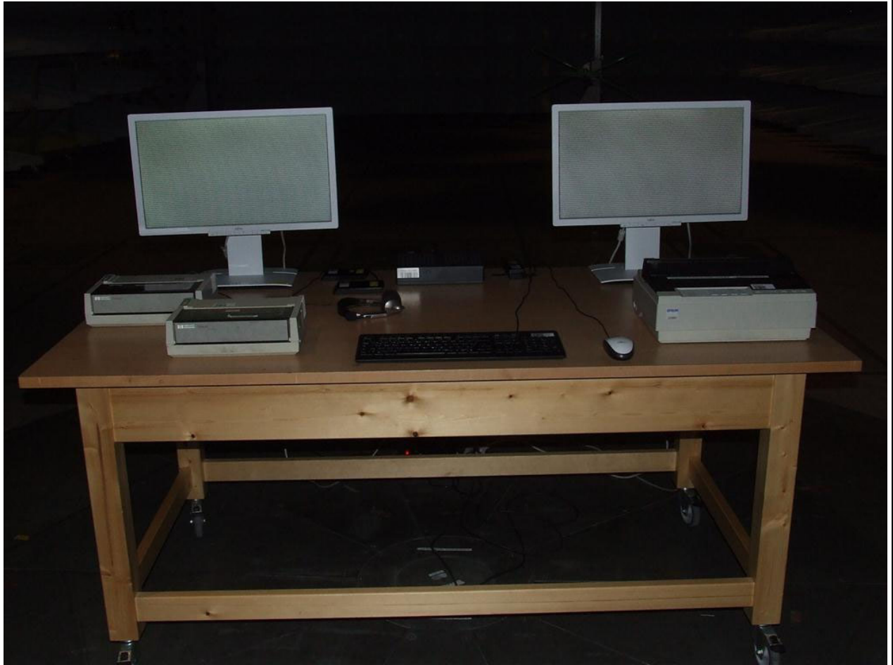
Figure 1 : Test set up Radiated Disturbance Emission - rear view
