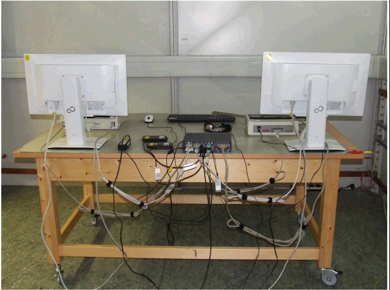
Figure 2 : Test set up for Electrostatic Discharge Immunity - rear view
