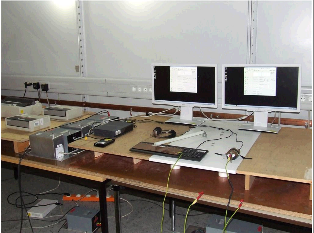
Figure 1 : Test set up for Conducted Disturbances Immunity - front view
