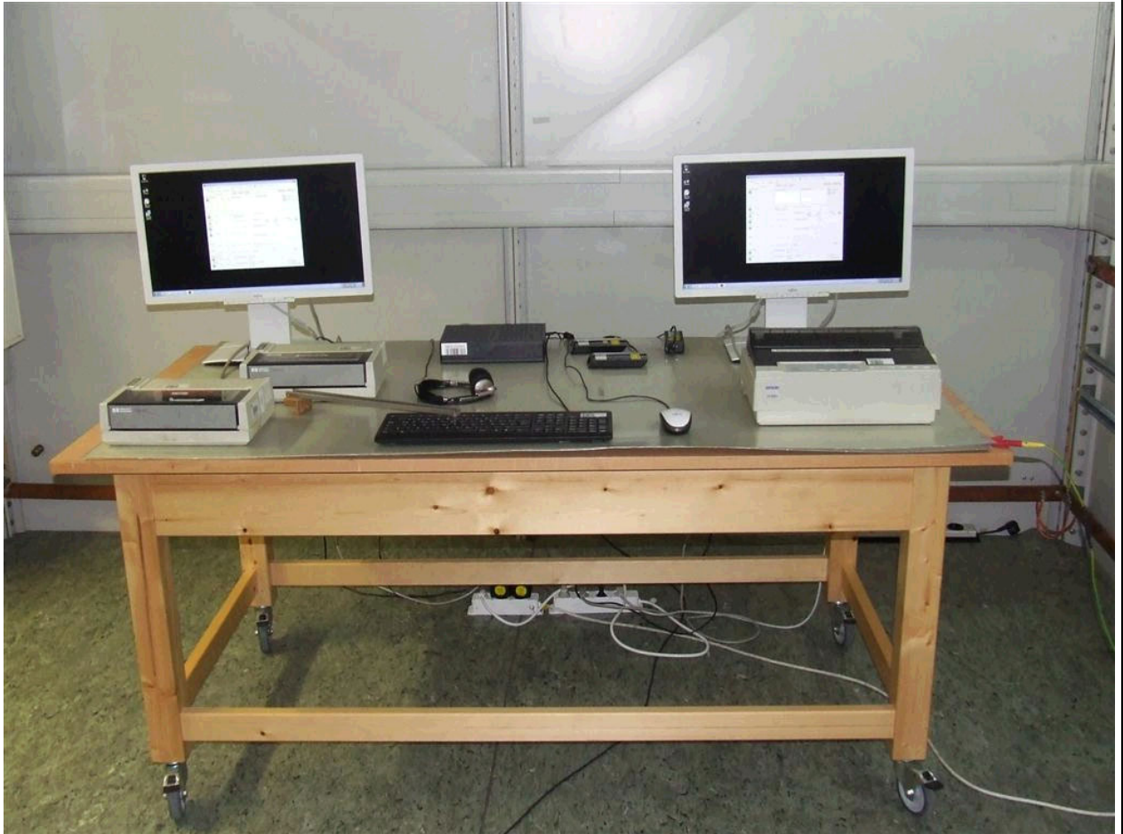
Figure 1 : Test set up for Electrostatic Discharge Immunity - front view
