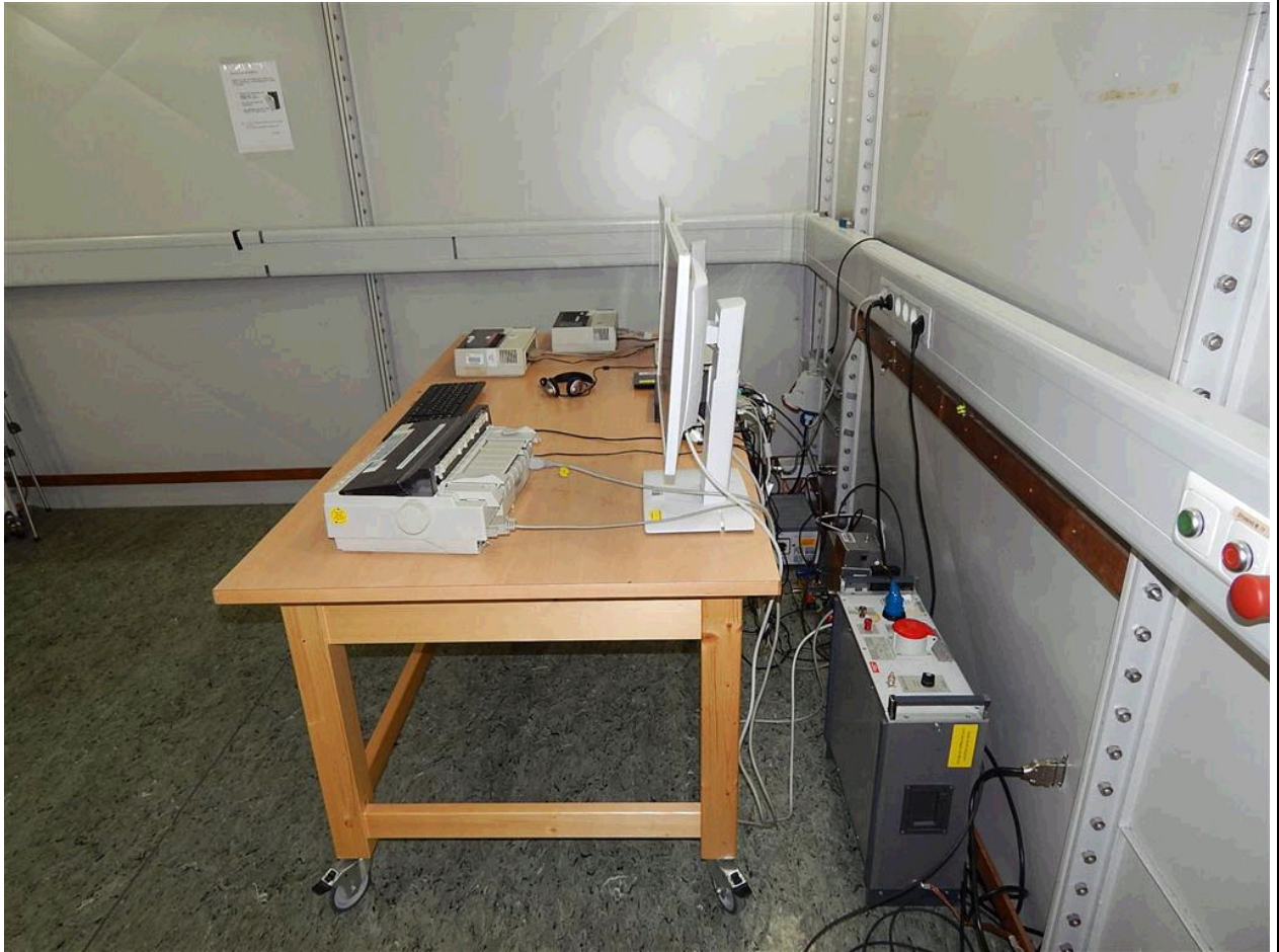
Figure 2 : Test setup for Conducted Disturbances Emission - side view
