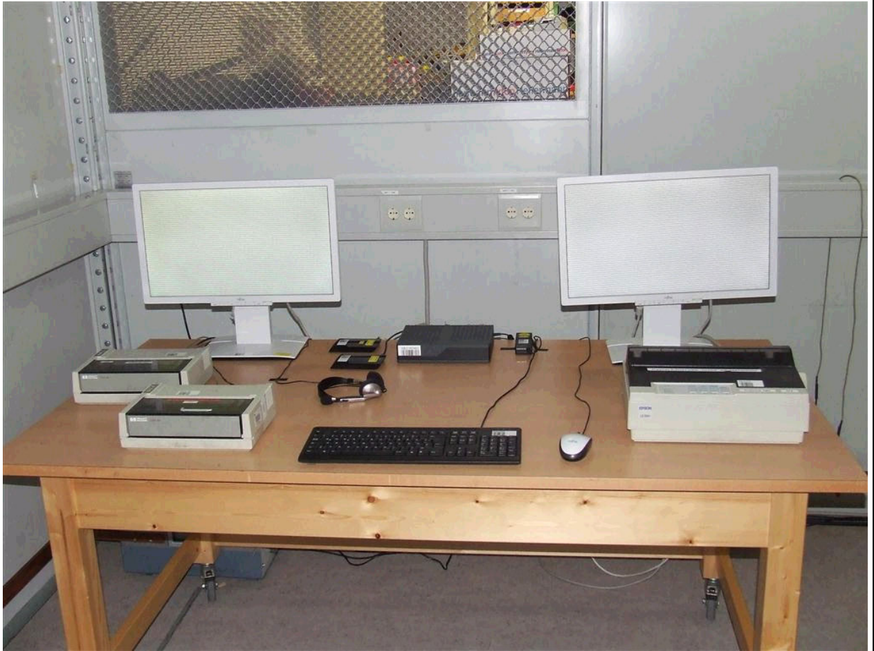
Figure 1 : Test setup for Conducted Disturbances Emission - front view
