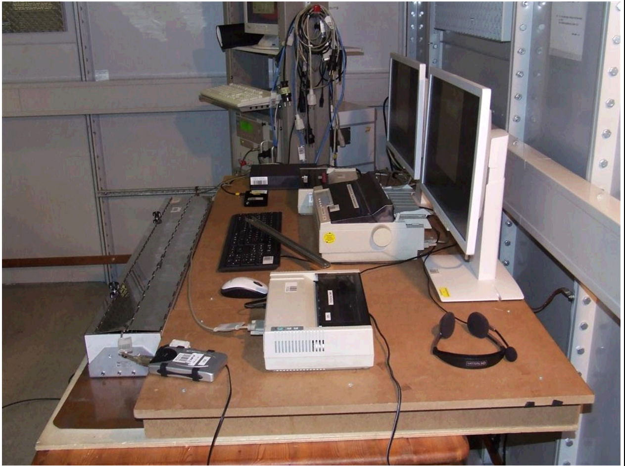
Figure 2 : Test set up for Electrical Fast Transient Immunity, Burst - side view
