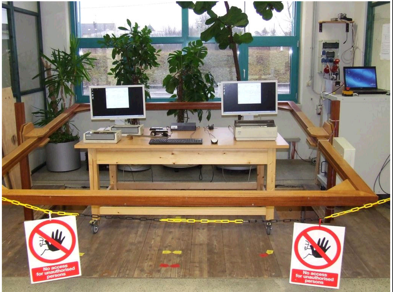
Figure 3 : Test set up for Immunity to power frequency magnetic field - z axis
