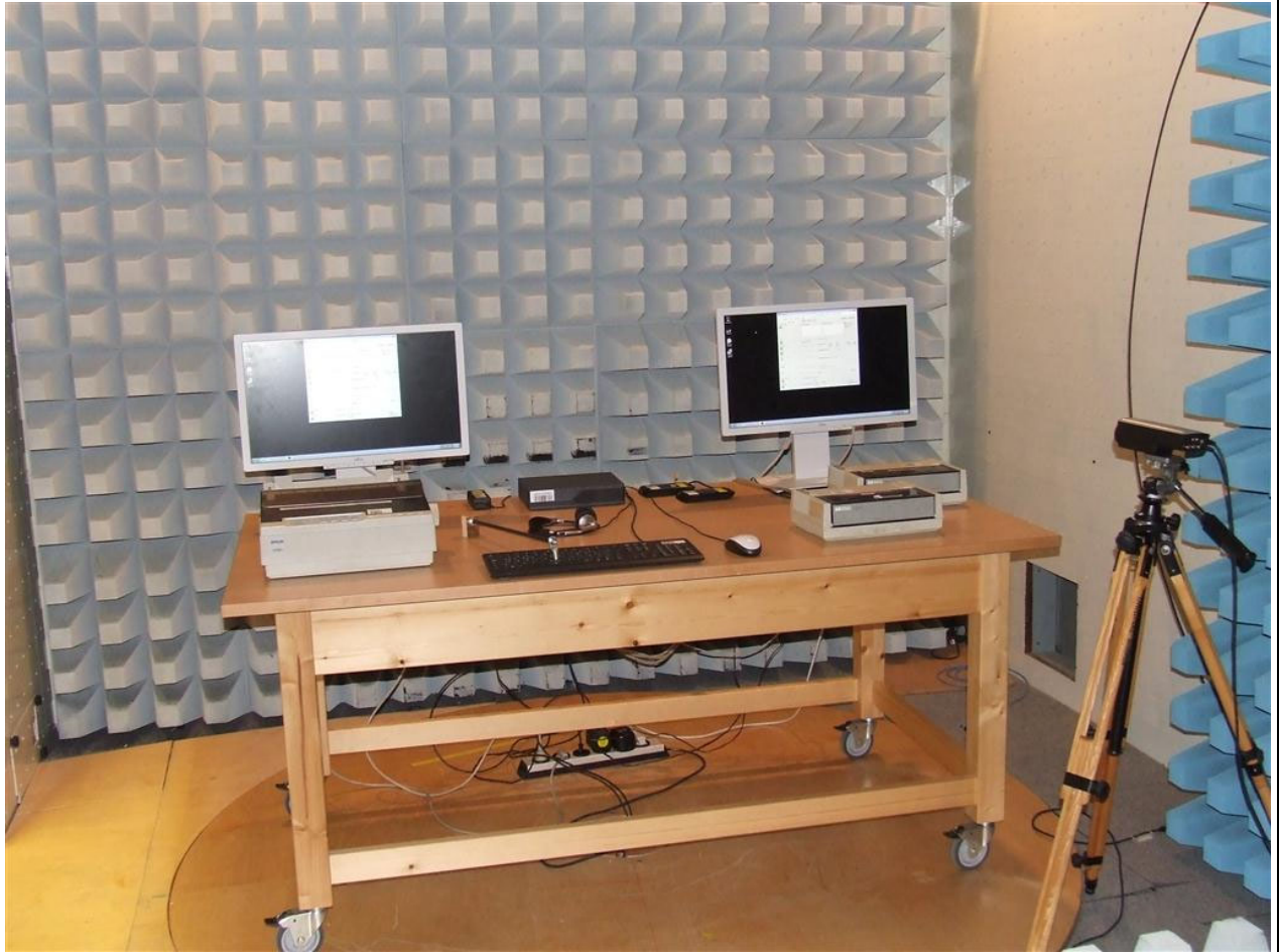
Figure 1 : Test set up Radiated Electromagnetic Field Immunity - front view
