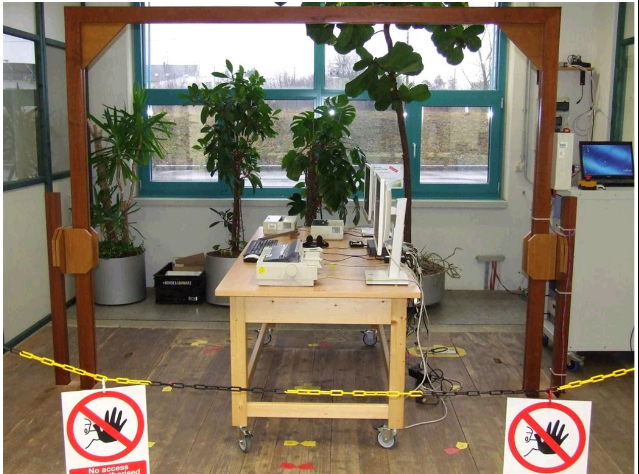
Figure 1 : Test set up for Immunity to power frequency magnetic field - x axis
