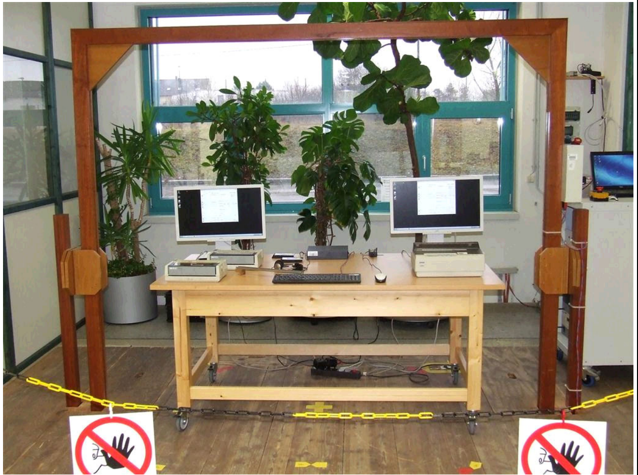
Figure 2 : Test set up for Immunity to power frequency magnetic field - y axis
