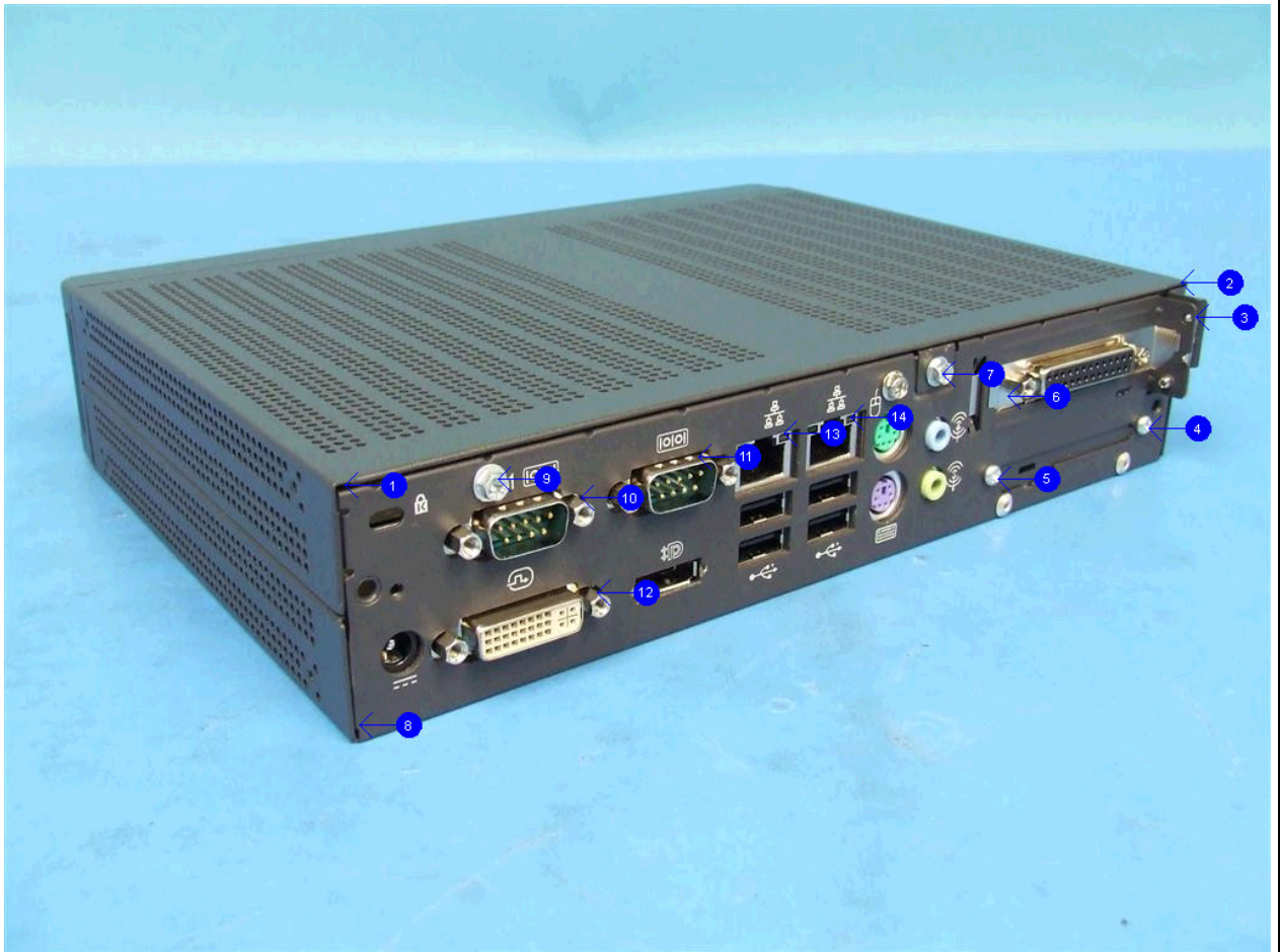
Figure 4 : Test set up for Electrostatic Discharge Immunity - test points rear. Air discharge
