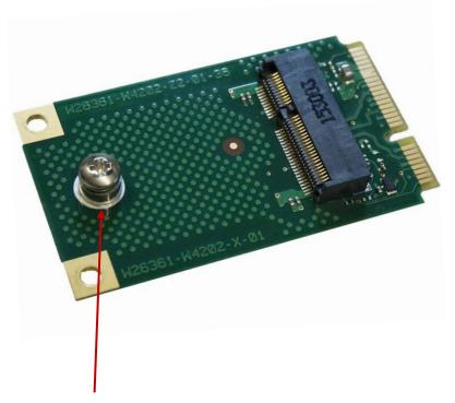
**Spacer (Nut) and M3 Screw for installing the 30mm M.2 Module**(cross-head screw M3 x 3.5; bolt head Ø = 4.5mm)
