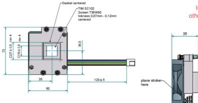
Important Note: Insulating foil of backplate must NOT be removed, otherwise mainboard may be damaged due to possible shortcut.
