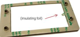
Important Note: Insulating foil of backplate must NOT be removed, otherwise mainboard may be damaged due to possible shortcut.
