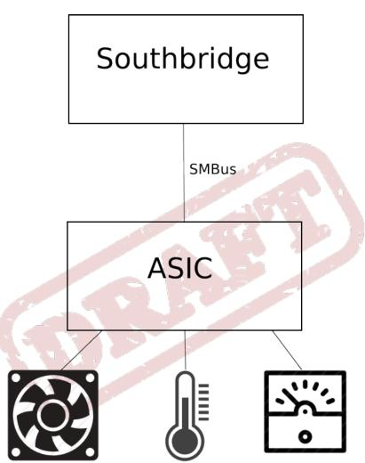
The ASIC is connected to the southbridge using an SMBus (System Management Bus) which is usually an I2C bus. The ASIC is capable of monitoring the fan speeds, the thermal sensors and the voltages of your systemboard.
