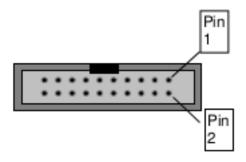
Pinout of the GPIO connector
