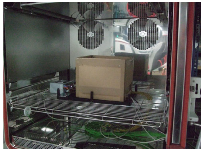
Picture no. 6: EUT in climatic cabinet
