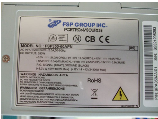
Picture no. 3: PSU type label
